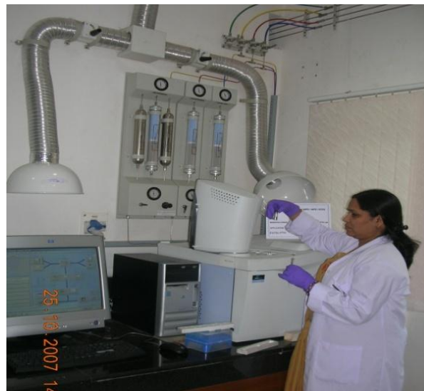
Pesticides Analysis at Gas Chromatograph (GC-ECD/ECD)
