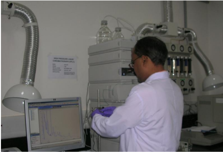
Perkin Elmer High Performance Liquid Chromatograph (HPLC) with RID, FLD, DAD and IC Detectors
